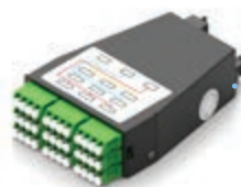
36 Fibre cassette with 3 x 12 rear MTP®/MPO adaptors and 36 LC/A adaptors
